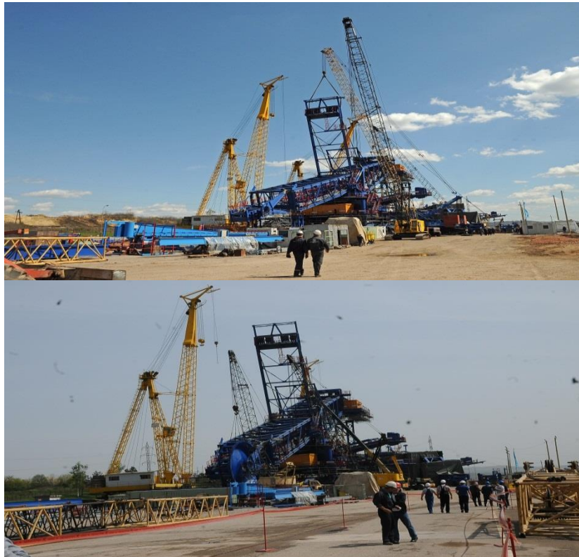
Figure 3. final assembly newest bucket wheel excavator latest generation technical, heavy mining system in the mounting plot in EPS, Branch RB "Kolubara" (2016).
